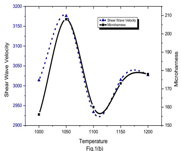
**Figure 1 :** Variation in Ultrasonic Velocity and hardness.
