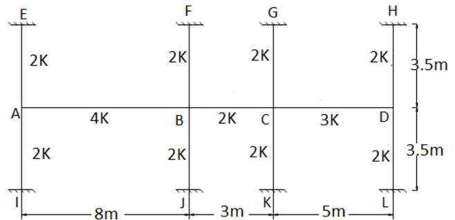
Figure 1: A substitute frame taken for example
