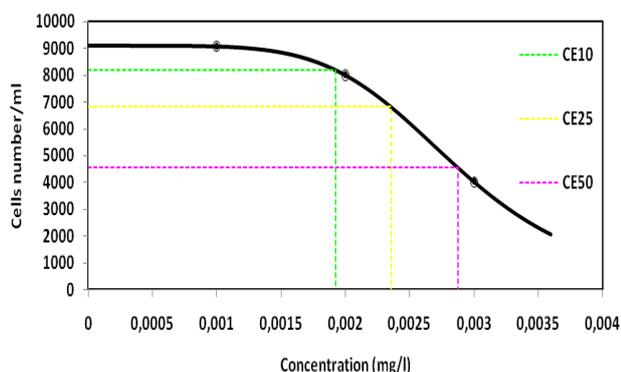
**Figure 3 :** Median Effective Inhibitory Concentration (EC50 expressed in mg/l) of Thiram using growth of *Paramecium sp.*
