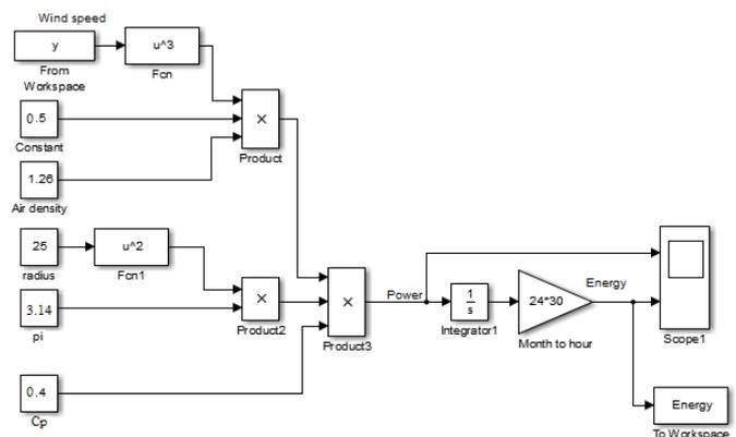
Figure 2 : The Block diagram for wind Turbinr
