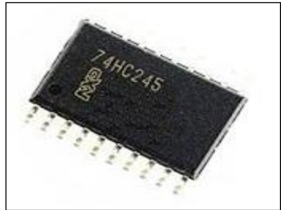
Figure.5 74HC245 (Communication chip)
