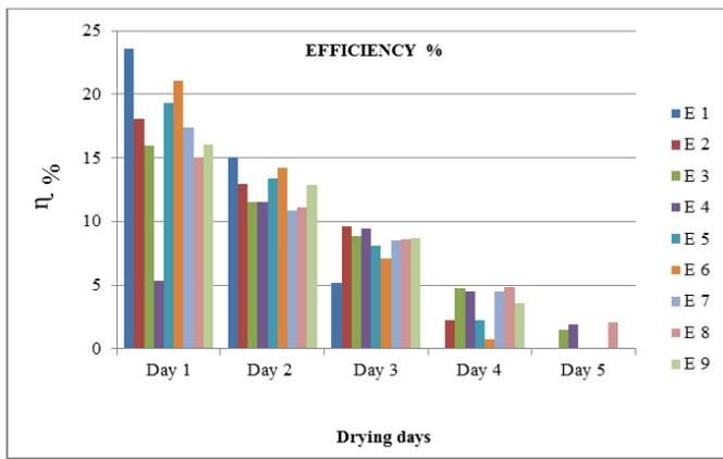
**Figure 3:** Per Day Efficiency of Solar Tunnel Dryer
