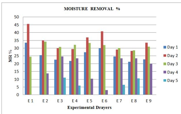
**Figure 4.** Per Day Moisture Removal for Different Experiments
