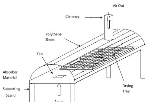
Figure 1: Schematic of Solar Tunnel Dryer
