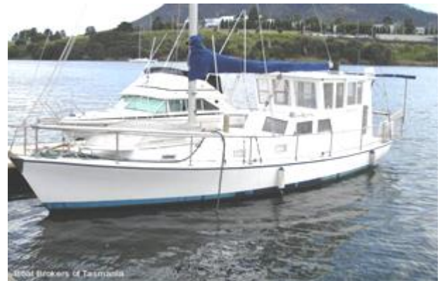
Figure 5: Ferrocement used in making boats
