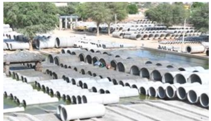
Figure 6: Ferrocement used in sewage pipes
