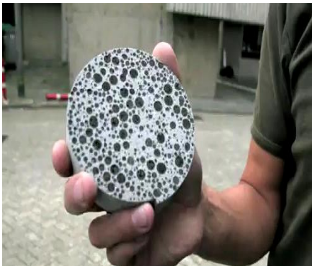
Figure 1: A sample of bacterial concrete
