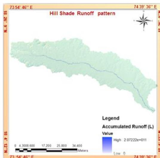
Figure 11: Accumulated Runoff (L) Drapped over Sun-Illuminated Topography
