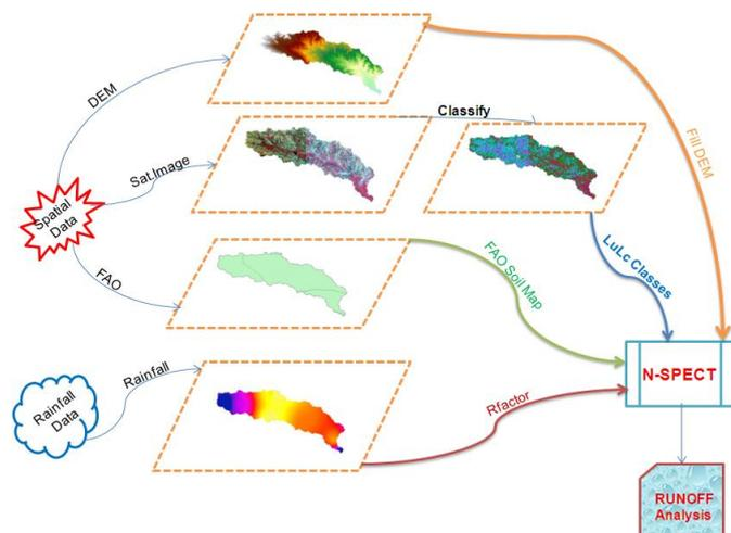
**Figure 8:** Methodology Applied for N-SPECT Model
