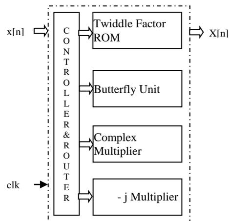
Figure 5 : High Level Block Diagram – Design 1
