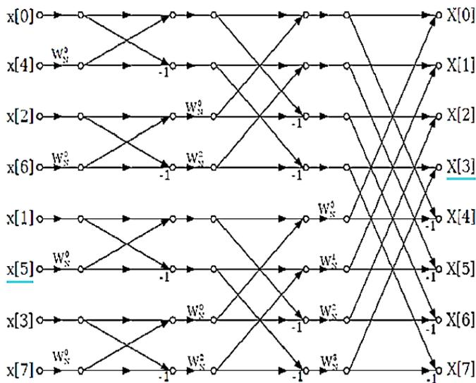
**Figure 2:** DIT-FFT radix-2 operation diagram
