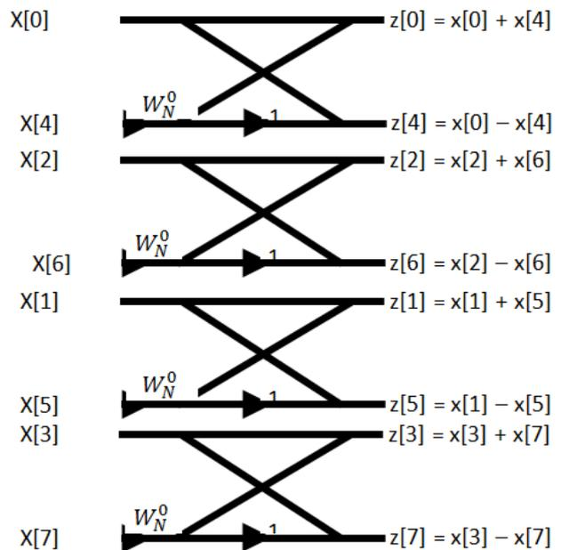
**Figure 3 :** Stage 1 of butterfly structure
