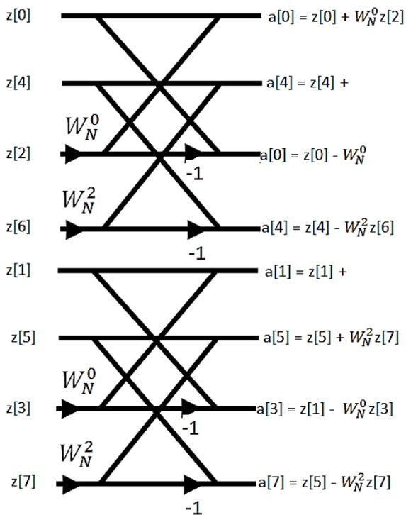
Figure 4 : Stage 2 of butterfly structure
