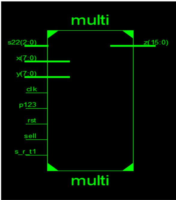
Figure 4: RTL View of Urdhwa Multiplier using Barrel Shifter
