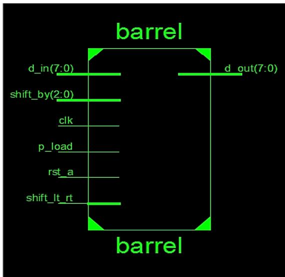
Figure 2: RTL view of barrel Shifter
