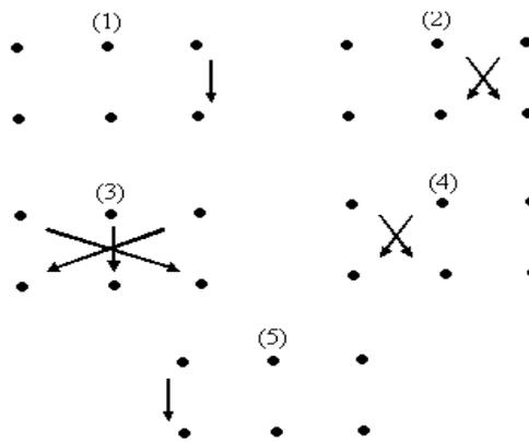
**Figure 1** : Multiplication procedure using “Urdhva - Tiryagbhyam” sutra
