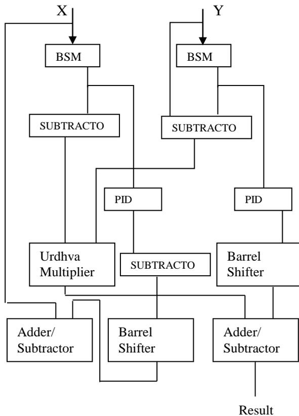
Figure 3: Urdhva Multiplier using Barrel Shifter
