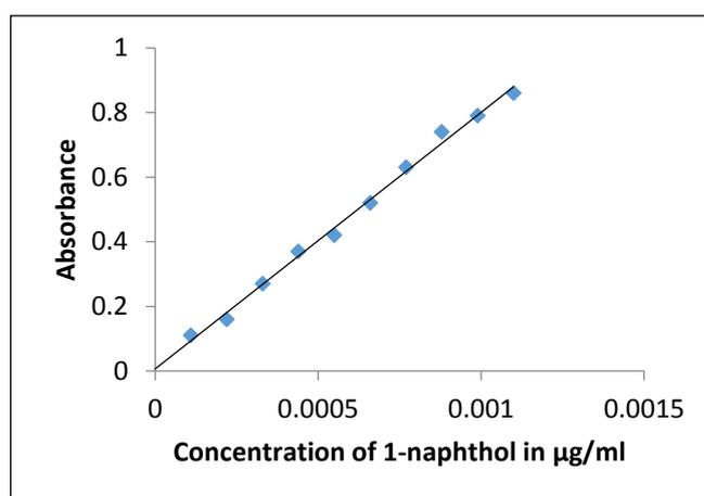
Figure 1: Calibration curve for 1-naphthol – NPBHA complex
