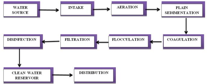
Figure 3 : Flowchart –Water Treatment Plant
