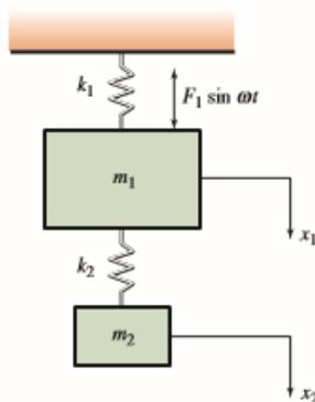
**Figure 1 :** Two DoF Undamped Dynamic Vibration Absorber
