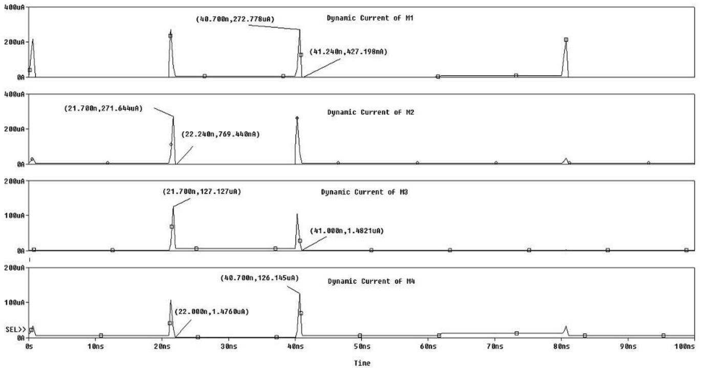
**Figure 3:** The waveform for dynamic current in 8T SRAM cell
