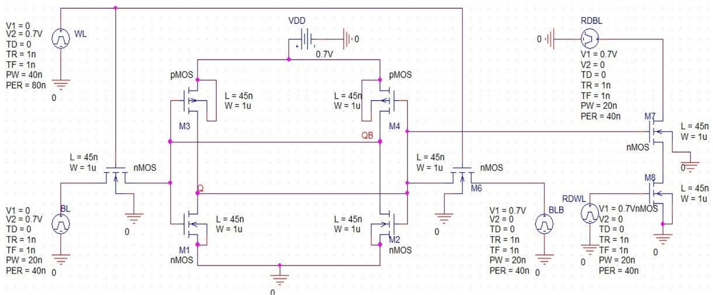
**Figure 1:** The Schematic of 8T SRAM Cell
