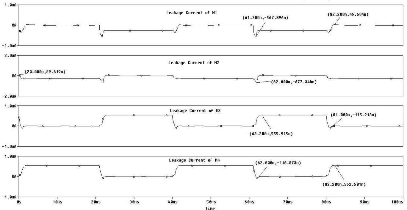
**Figure 4:** The waveform for leakage current in 8T SRAM cell
