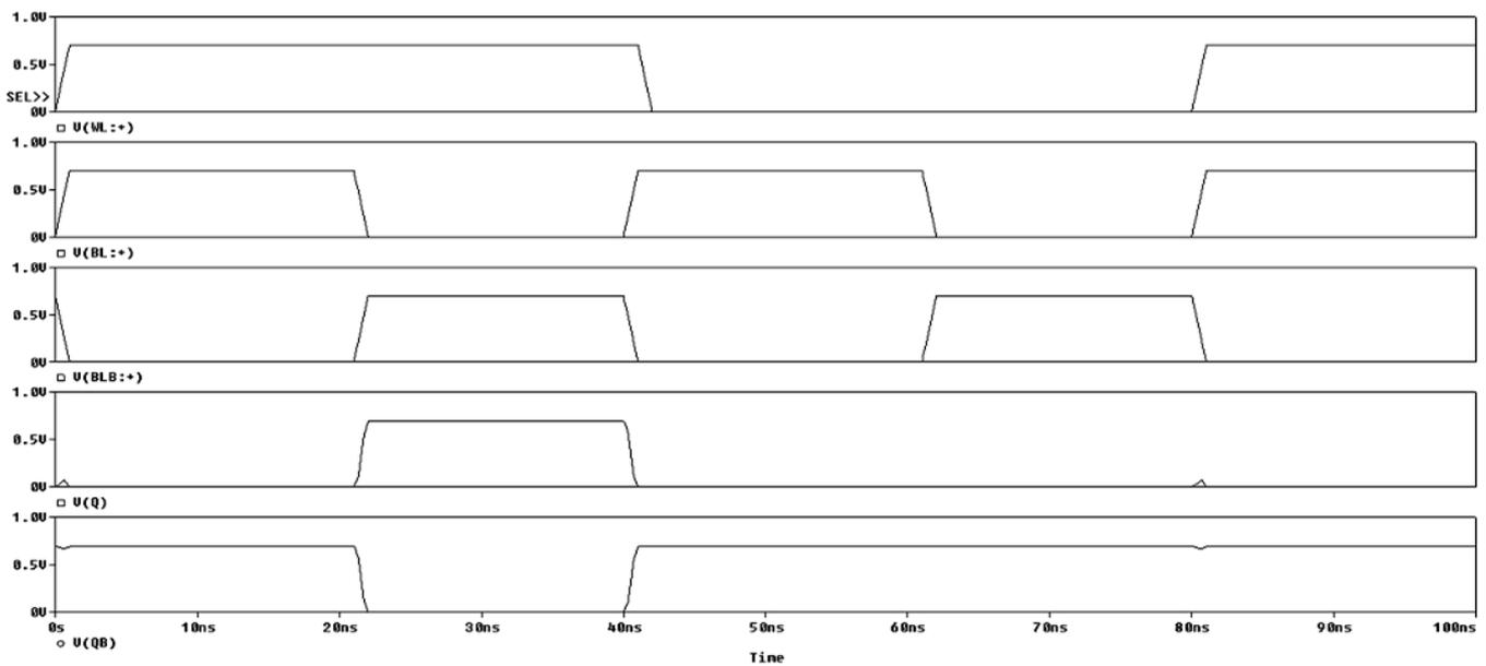
Figure 2: The waveform for write operation in 8T SRAM cell
