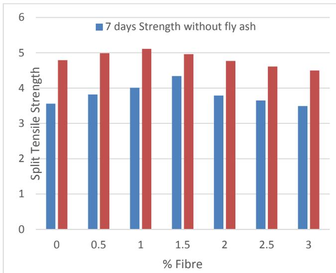
**Figure 4 :** Tensile Strength at 7 and 28 days without Fly Ash
