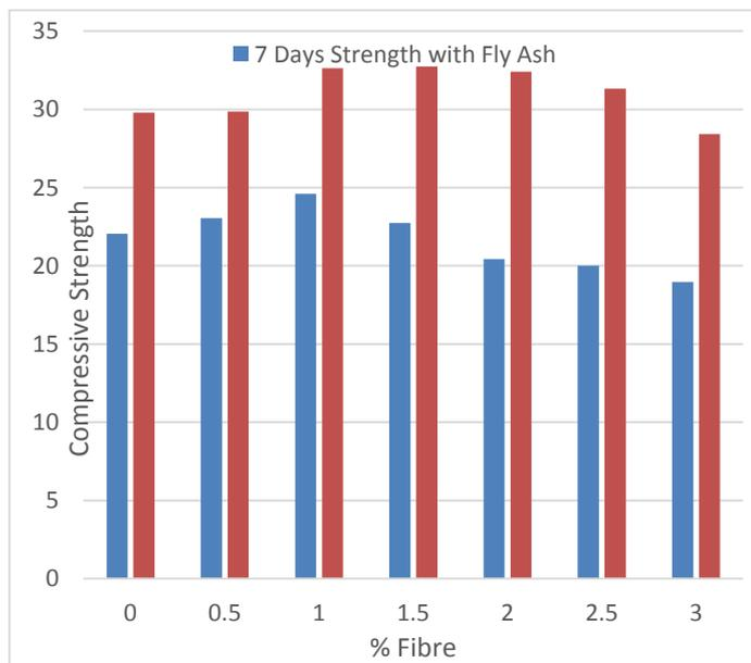
**Figure 1 :** Compressive strength at 7 and 28 Days with Fly Ash
