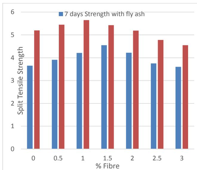
**Figure 3 :** Tensile Strength at 7 and 28 days with Fly Ash
