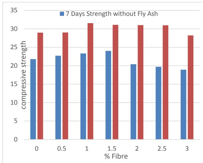
**Figure 2 :** Compressive strength at 7 and 28 days without Fly Ash
