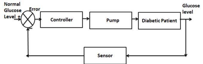
**Figure 1** : Block diagram of Glucose Insulin regulation system<sup>[3]</sup>
