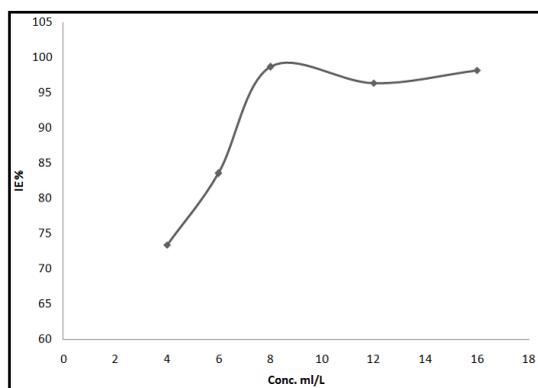
Figure 2: Relationship between concentrations of Sumac extract and inhibition efficiency.
