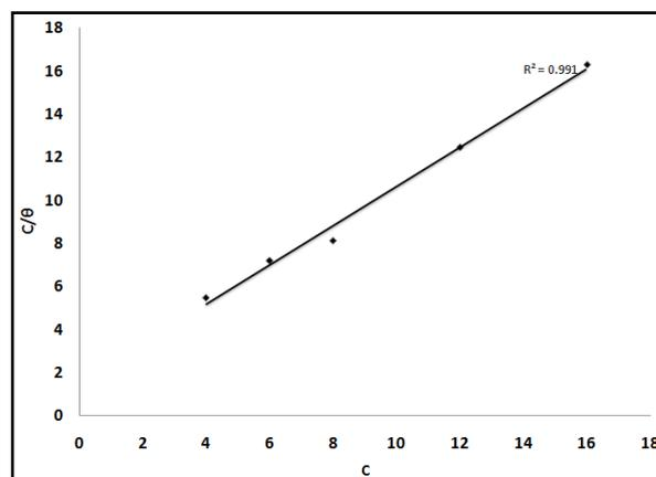
Figure 3: Langmuir adsorption plot for steel in seawater in the presence of Sumac extract with five concentrations.
