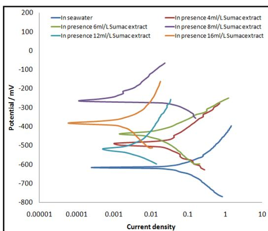
Figure 1: Tafel plots of steel in uninhibited and inhibited seawater at room temperature.
