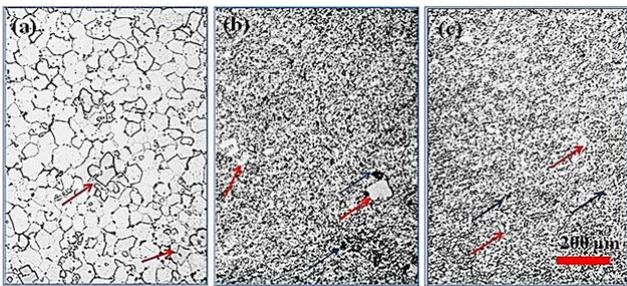
**Figure 5 :** Illustration of optical micrographs of studied alloy at different conditions: (a) T4 (no FSP), (b) T4+FSPed, (c) T4 + FSPed +Aged at 140 oC/2h.
