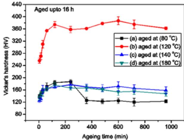
**Figure 1** : Illustration of artificial ageing curves of studied alloy at different temperatures: (a) aged at  $80^\circ\text{C}$ , (b) aged at  $120^\circ\text{C}$ , (c) aged at  $140^\circ\text{C}$ , (d) aged at  $180^\circ\text{C}$ .
