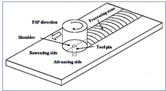
**Figure 2** : The diagram of friction stir processing set-up.
