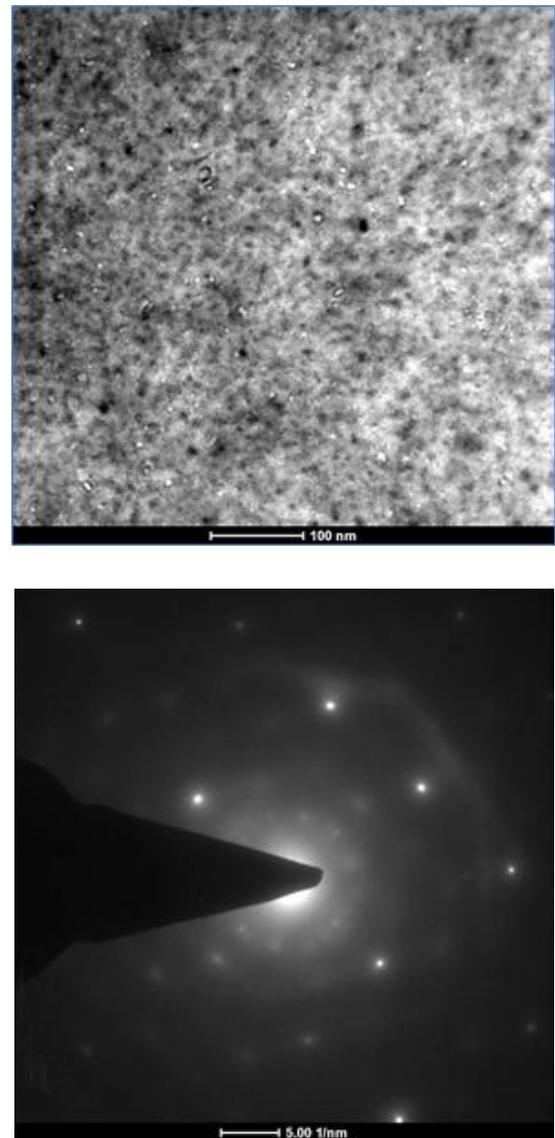
**Figure 3 :** The TEM micrograph with CCD pattern at  $T_6$  condition (aged at 100 oC/6h).
