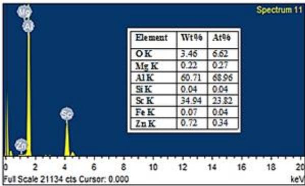
**Figure 4 :** The SEM with EDX analysis of T4 + FSPed alloy.
