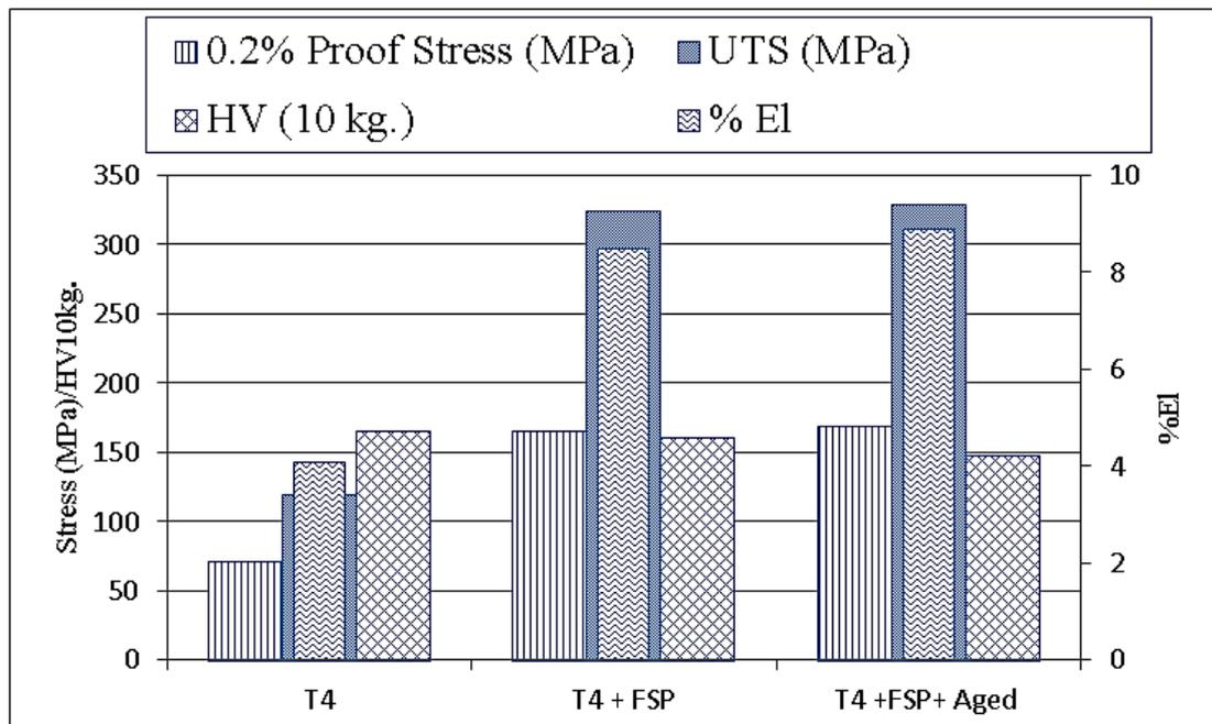
**Figure 7 :** The bar diagrams represented the mechanical property of studied alloy after double passes FSPed at different stages.
