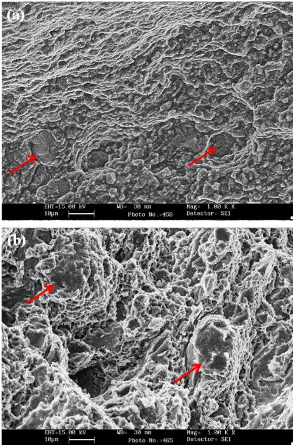
**Figure 6 :** The illustration of SEM tensile fracture surfaces after (a) T4+FSPed, (b) T4+FSPed+Aged at 140 oC/2h condition
