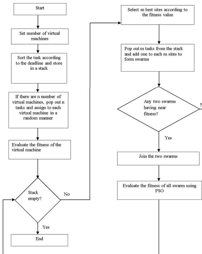
**Figure 1 :** Flow chart of the HBPSO algorithm for task scheduling and resource allocation
