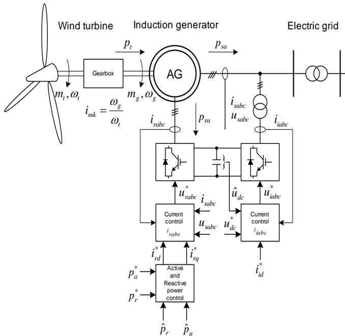
**Figure 1 :** Wind turbine Active control system with DFIG
