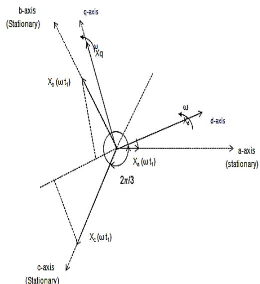
**Figure 3 :** Decomposition of space vector  $\vec{x}$  into dq rotating reference frame.
