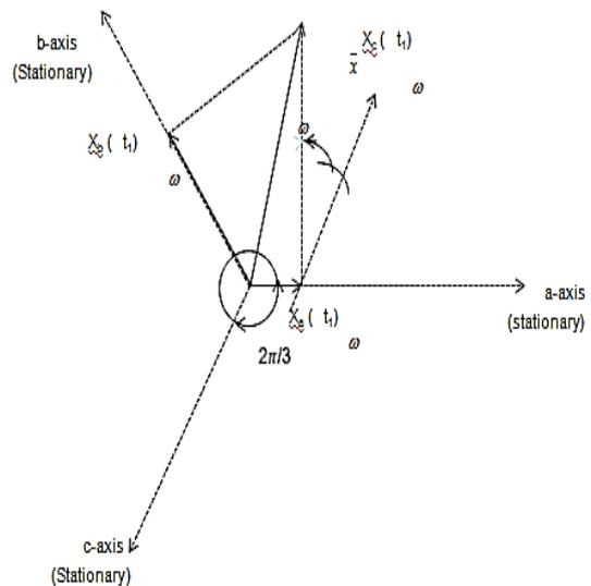
**Figure 2 :** Space vector  $\vec{x}$  and its three phase variables  $x_a$ ,  $x_b$  and  $x_c$ .
