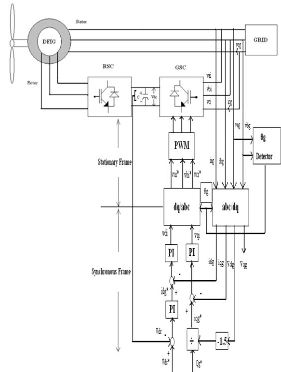
Figure 4 : control scheme of grid side converter
