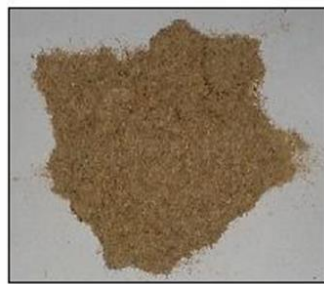
Figure 2 : 212 \mu m fiber
