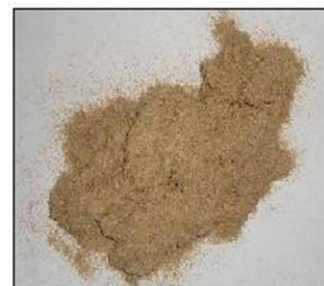
Figure 4 : 106 \mu m fiber
