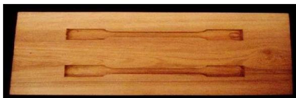
Figure 6 : Wooden Die block for tensile test
