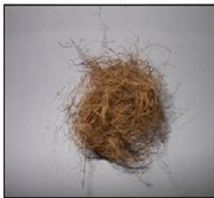
Figure 1 : Palm Fiber (0.5 mm)
