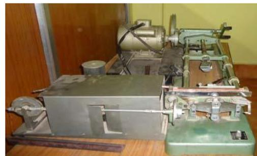
Figure 7 : The Tensometer
