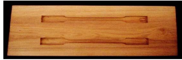
Figure 6 : Wooden Die block for tensile test
