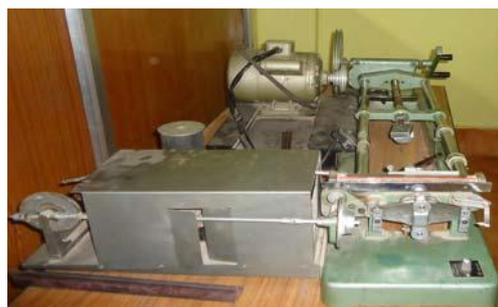
Figure 7 : The Tensometer
