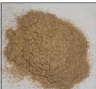
Figure 3: 150 \mu m fiber
