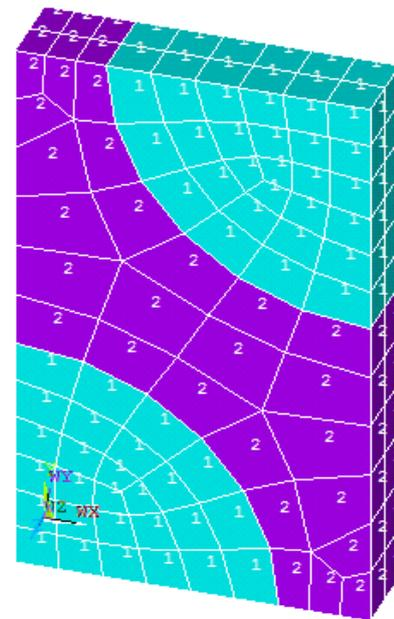
**Figure 2 :** Meshed model of representative volume element
