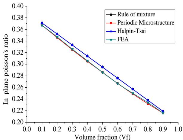
**Figure 7 :** In plane Poisson's ratio validation with different volume fraction.
