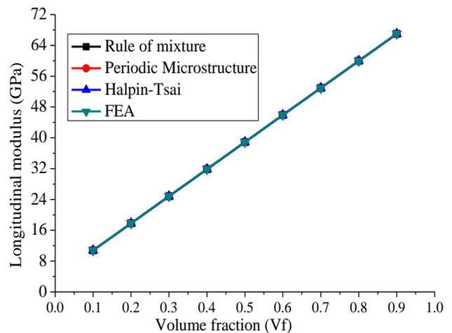
**Figure 5 :** Longitudinal modulus validation with different volume fraction
