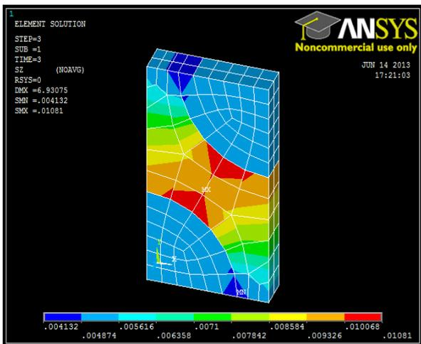
**Figure 3 :** Counter of stress in representative volume element
