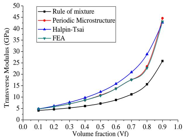
**Figure 6 :** Transverse modulus validation with different volume fraction
