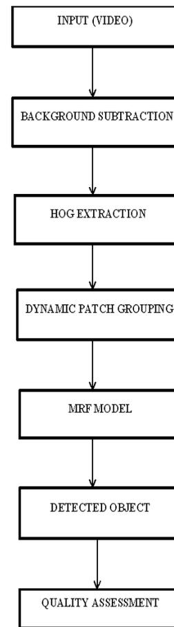
**Figure 1** : shows the flow diagram of the MRF based abnormal detection in video.
