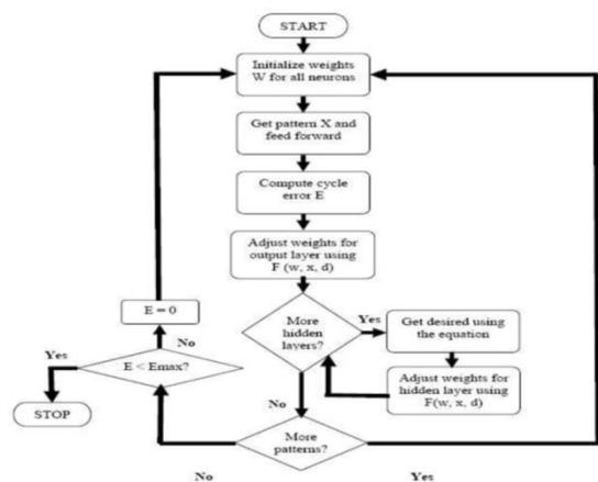
**Figure 4.** Flowchart showing working of BPA
