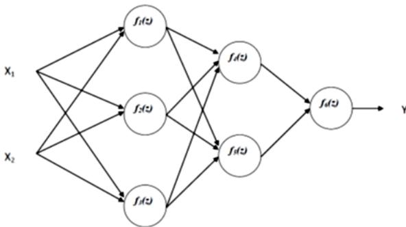
**Figure 3.** Three layer neural network with two inputs and single output
