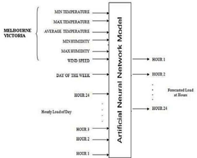
Figure 5. Input-Output Schematic for Load Forecasting.
