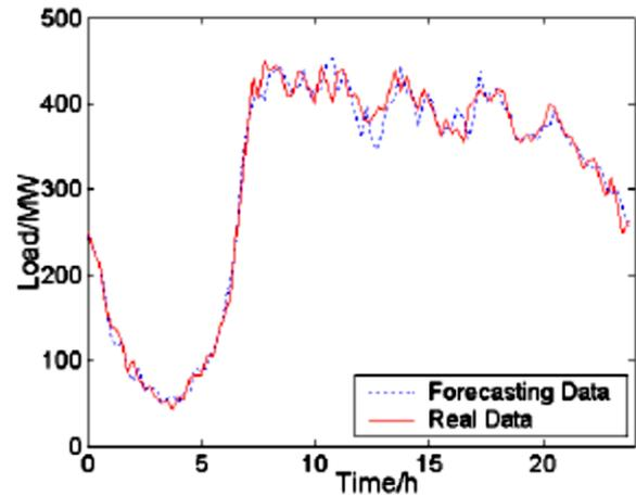
Figure 2. Real load data and the corresponding forecasting data
