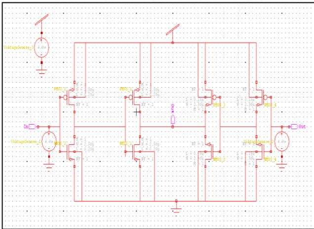
**Figure 7 :** Schematic for Binary to Quaternary Converter Circuit
