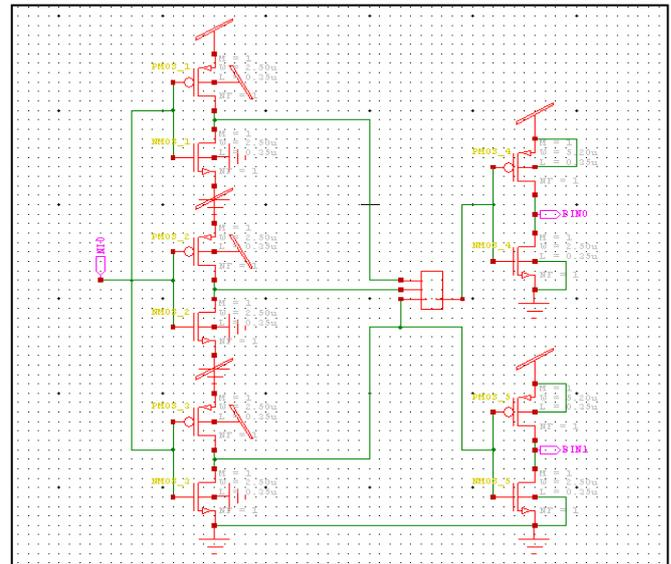
Figure 4 : Schematic for Quaternary to Binary converter Circuit
