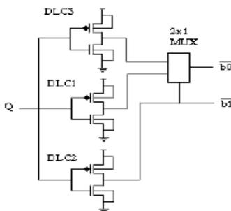
Figure 3 : Quaternary to Binary converter circuit
