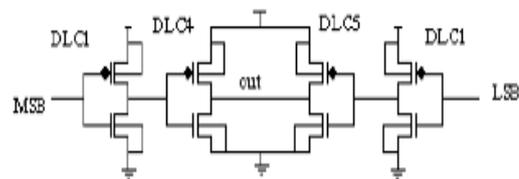
Figure 6: Binary to Quaternary converter circuit
