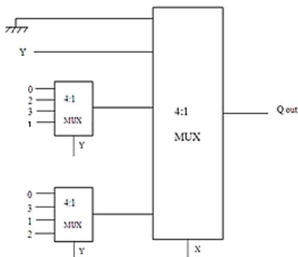
Figure 12: Logic diagram for GF (4) multiplier
