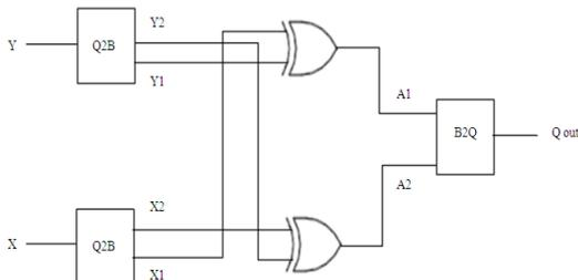
**Figure 9 :** Logic diagram for GF (4) adder
