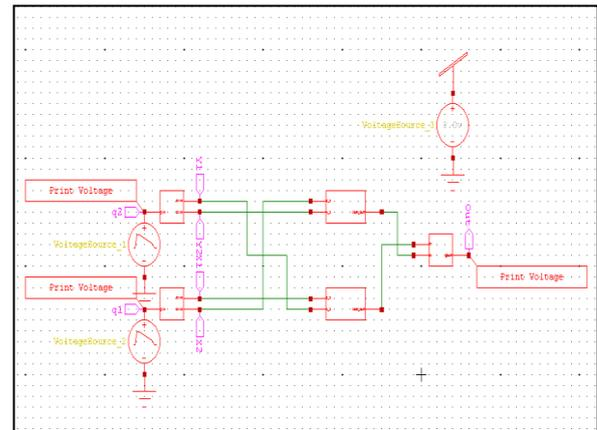
**Figure 10:** Schematic for GF (4) Adder
