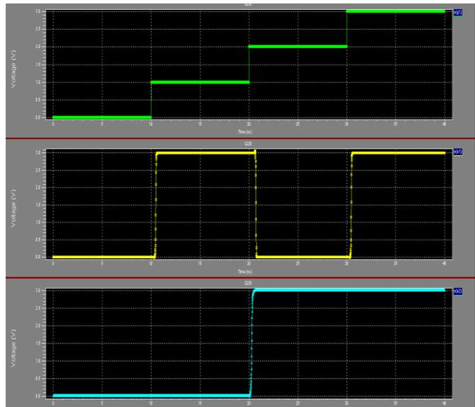
Figure 5 : Simulation result of Quaternary to Binary Converter Circuit
