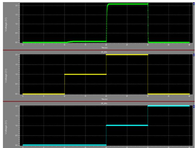
Figure 14: Simulation result of GF (4) multiplier
