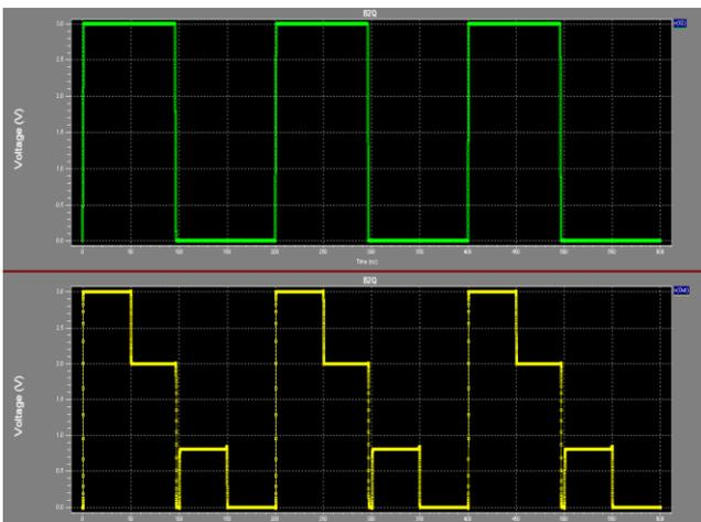
**Figure 8:** Simulation result of Binary to Quaternary Converter Circuit
