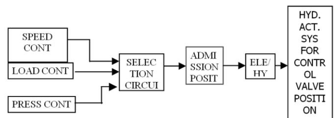
In Mechanical Hydraulic Governing, we are just opening / closing the secondary oil drain thereby varying the HP /IP control valves position. Hence Load will be varying according to the Frequency and Drum Pressure. But in EHG Load is maintained constant to the set value by providing various closed loop control systems. In EHG we have 3 control loops namely
