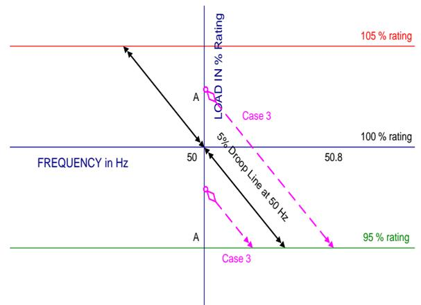
When the frequency rises from 49 to 50 Hz, Load reduction signal should be blocked.
