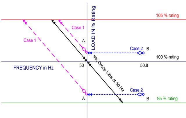
During the frequency rise from 50 Hz to a higher value, Load reduction signal is released up to 5 % as per the droop characteristics.
