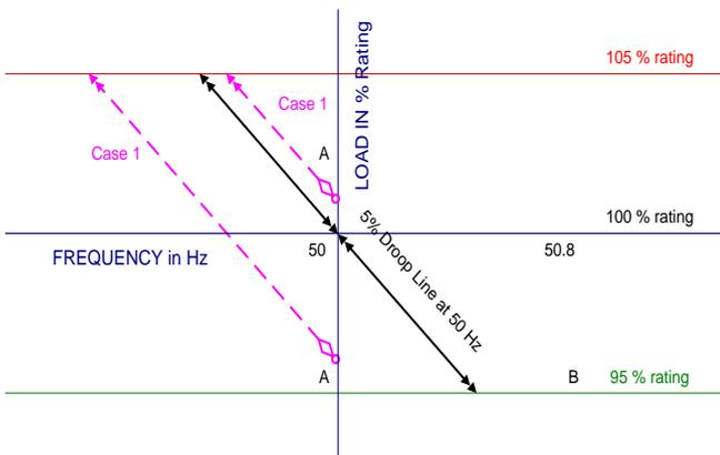
When the generator frequency is lowering towards 50Hz from a higher frequency, the load correction signal is blocked.
