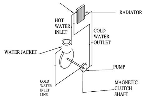
**Figure 2.** Water cooling system in two wheeler 4-stroke SI engine
