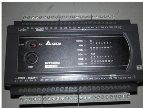
Figure 9. Digital PLC Board
