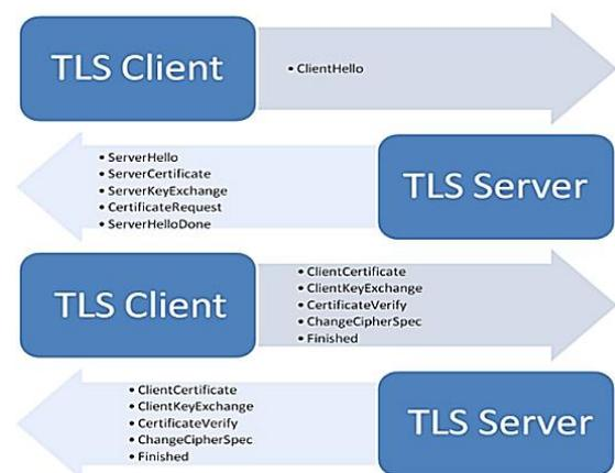
Figure 5. A typical flow of the TLS protocol
