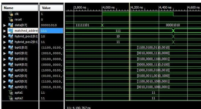
Figure 6. Output waveform for T-SRAM
