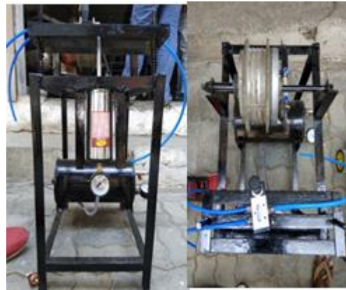
Figure 1. front and top view of compressed air generation using suspension of vehicle
