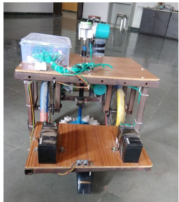
Figure 6. Hardware Model of Smart Floor Cleaner
