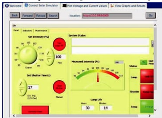
Figure 2: Remote control of the solar simulator using LabVIEW
