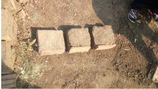
Figure 2. Tile faced mud block
