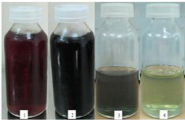
Fig.6 Freshly prepared blood red Copper solution (1), Black (2), Violet (3), Onset Oxidation (4)
