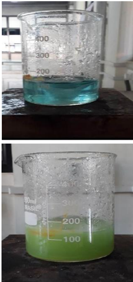
Fig 3 (a) Sky blue color obtained by adding copper nitrate and PVP (b) green color obtained after adding hydrazine hydrate
