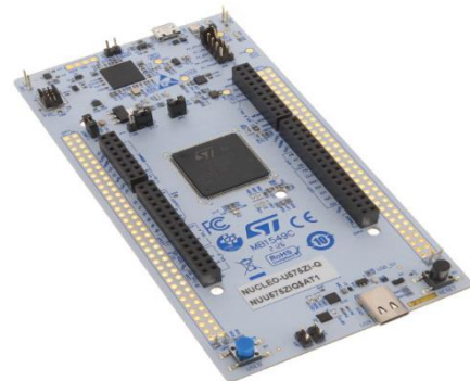
Fig 2. Introduction of STM32 Nucleo-U575ZI-Q Board
