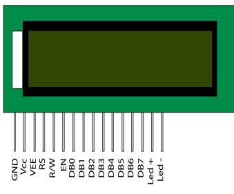
Figure 4. LCD Pinout (16\*2)
