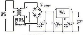
Figure 5. Power Supply Circuit
