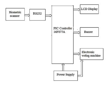
Figure 1. Block diagram of the proposed system
