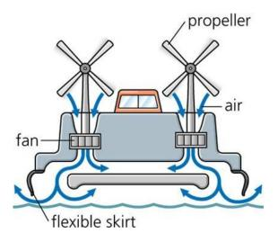
Figure 1. Schematic diagram
