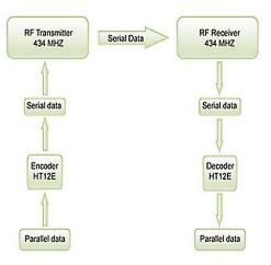
Figure 4. Transmission Diagram
