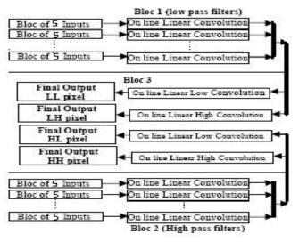
Figure 4. The decomposition matrix wavelet on line block diagram.
