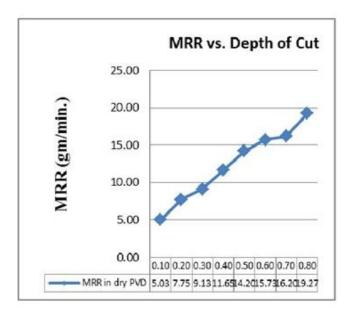
Figure 3(1). Effect of varying depth of cut on MRR
