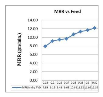
Figure 2. Effect of varying feed on MRR
