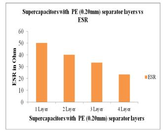
Figure 7: ESR of PE (0.20mm) separator layers of supercapacitor
