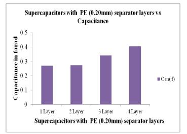
Figure 6 : Capacitance of PE (0.20mm) separator layers of supercapacitor
