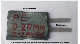
Figure 1: PE (0.20mm) separator two layers of super capacitor
