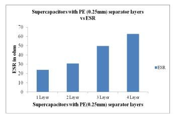
Figure 5: ESR of PE (0.25mm) separator layers of supercapacitor
