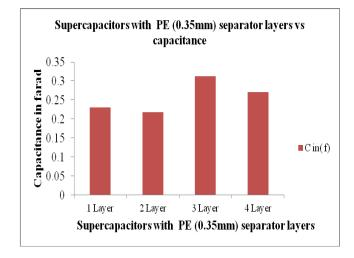
Figure 2: Capacitance of PE (0.35mm) separator layers of supercapacitor
