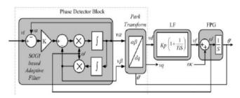
Figure 3. SOGI-QSG & Parks Transform based Phase Detector.
