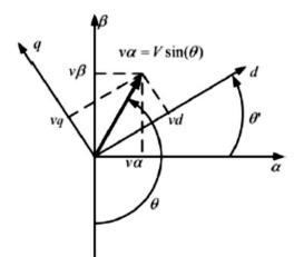
Figure 4. Vector diagram of SOGI-PARK based Phase detector
