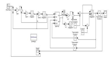
Figure 5. Simulation of SOGI PLL
