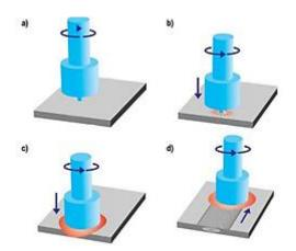
Figure 1. Schematic illustration of friction stir processing
