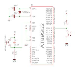
Figure 3. Circuit diagram of microcontroller circuit
