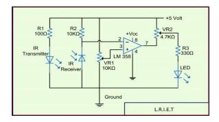
Figure 1. Circuit diagram of IR sensor
