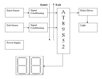
Figure 2. Block diagram of the Power saving
