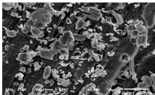
Figure 3b :- SEM of Sn 65 Al 20 Sb 5 Pb 5 Cd 5 alloy
