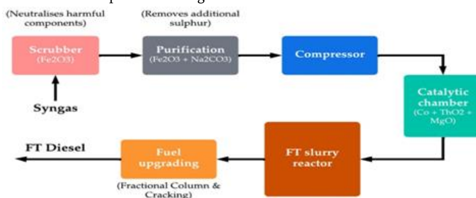
Fig 12. FT diesel production from syngas - Typical Fischer-Tropsch process
