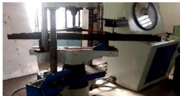
Figure3:Experimental Testing on Composite Leaf Spring.
