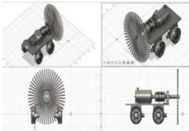
Fig 1. Design of prototype of AC Duct Cleaning Robot in Fusion-360
