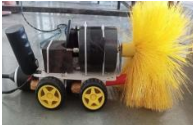
Fig 2. Actual Model of AC Duct Cleaning Robot
