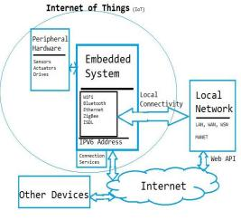
Figure1.Architecture of IOT
