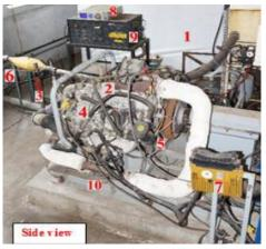
A single-cylinder, four-stroke, water-cooled diesel engine was used for the experiments. The engine was operated at a constant speed of 1500 rpm with three fuel blends:
