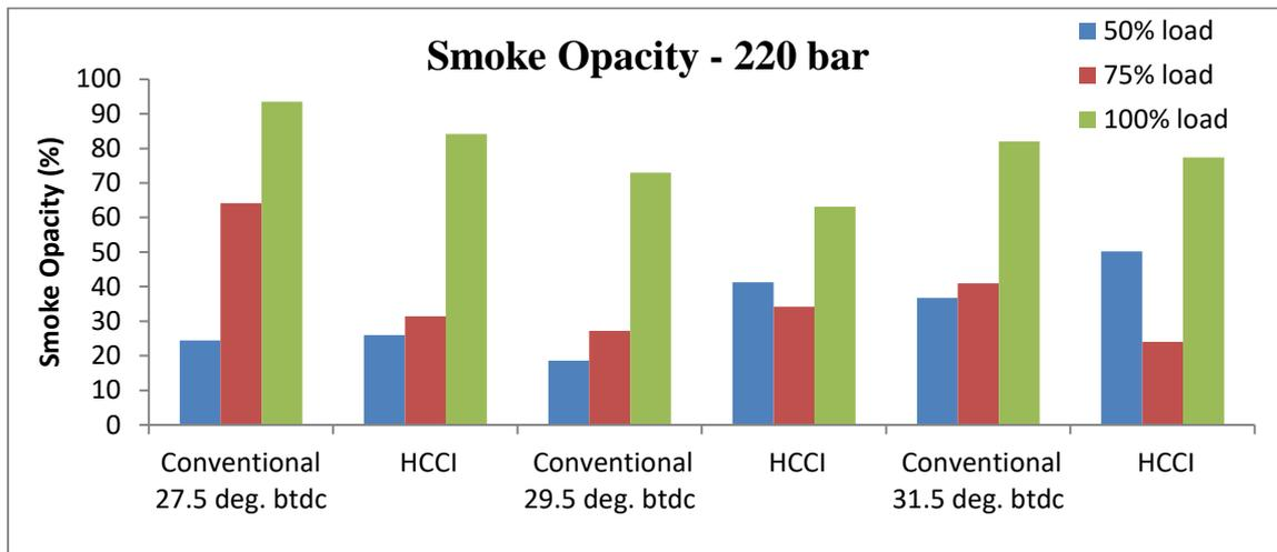
Figure 4.4.3 Smoke Opacity for conventional and vapour induction mode at different injection timings at 220 bar
