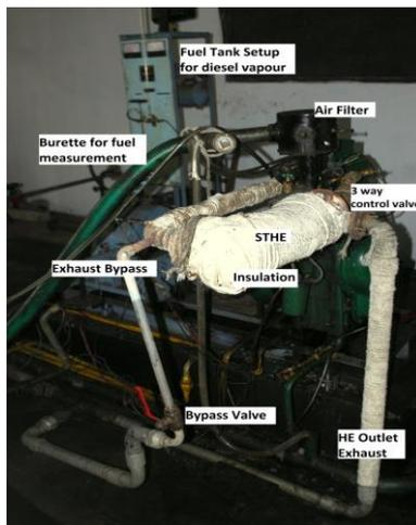
Figure 2.1 Experimental Setup for Vapour Induction
