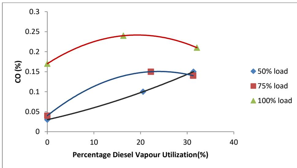
Figure 4.3.2. Effect of vapour induction on CO Emissions at 29.5 deg. btdc and 200 bar injection pressure
