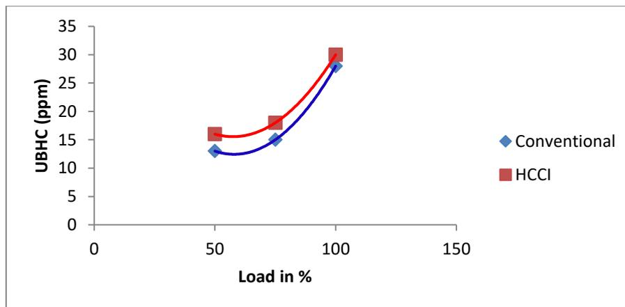
Figure 4.1.2 UBHC emissions at optimized vapour induction mode and conventional diesel injection mode at different loads
