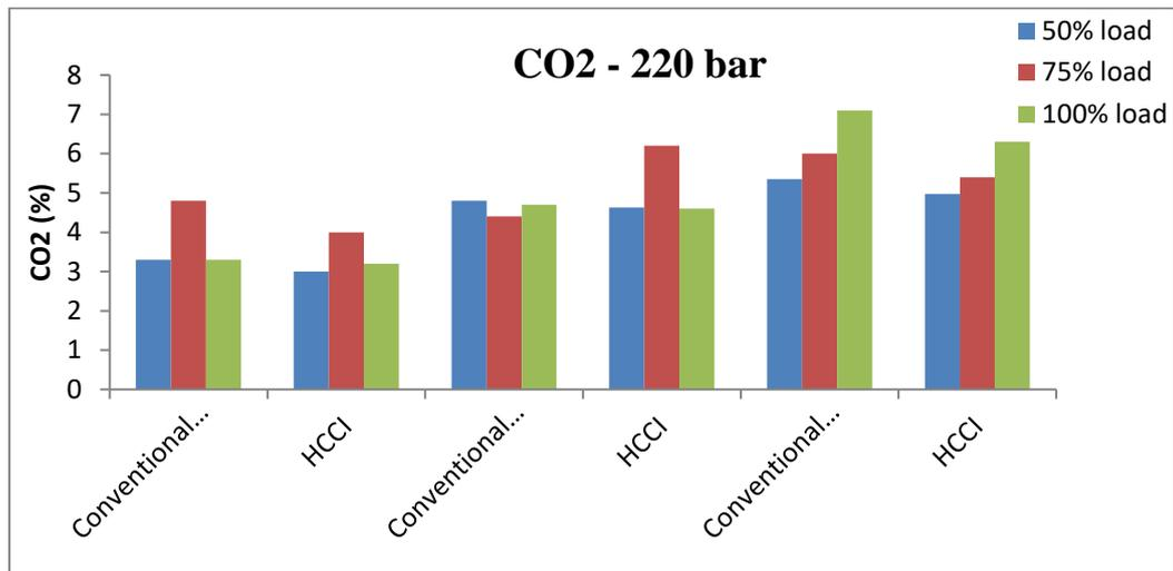
Figure 4.1.3 CO<sub>2</sub> emissions for conventional and vapour induction mode at different injection timings at 220 bar
