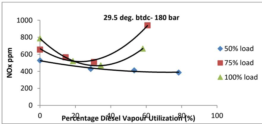
Figure 4.3.2 NOx variation with vapour induction at 29.5 deg. bt dc and 180 bar injection pressure.
