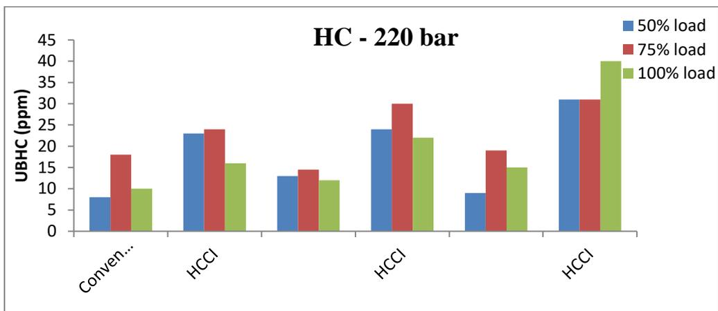
Figure 4.1.3 UBHC emissions for conventional and vapour induction mode at different injection timings at 220 bar
