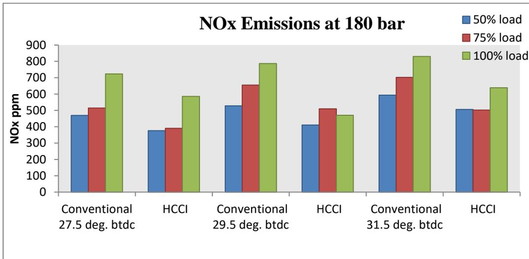
Figure 4.3.4. NOx emissions for conventional and vapour induction mode at different injection timings at 180 bar.
