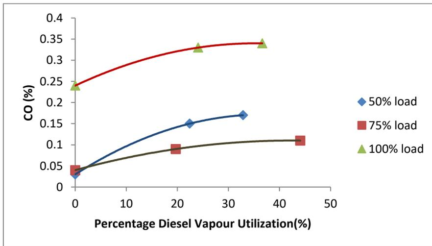
Figure 4.3.1 Effect of vapour induction on CO Emissions at 27.5 deg. btdc and 200 bar injection pressure
