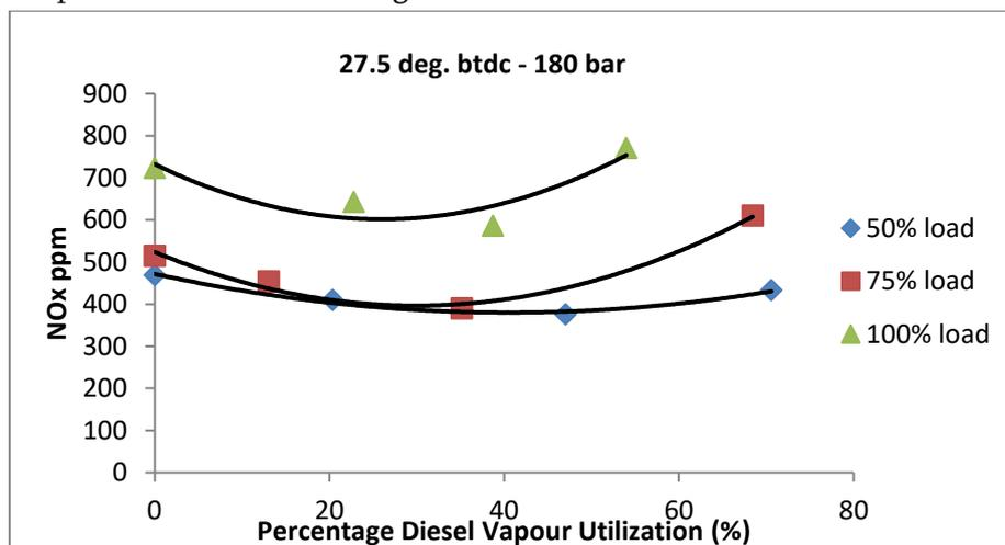
Figure 4.4.1 NO<sub>x</sub> variation with vapour induction at 27.5 deg. btdc and 180 bar injection pressure.
