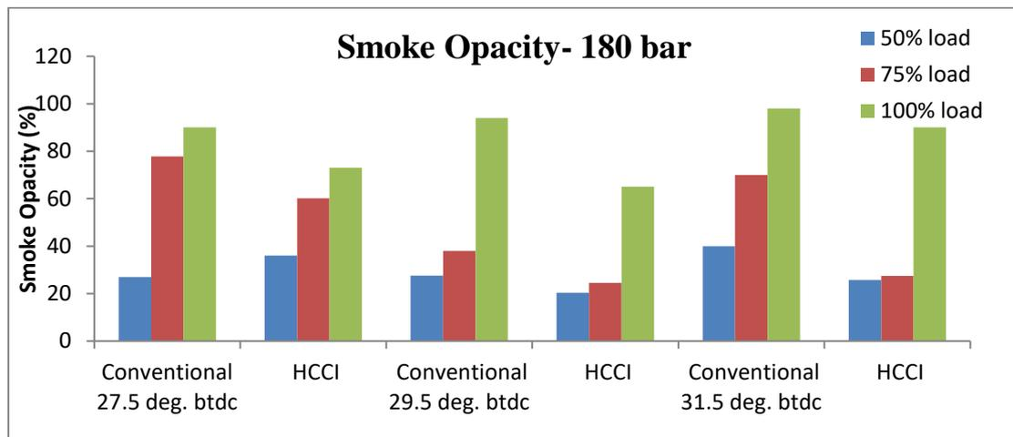
Figure 4.4.1 Smoke Opacity for conventional and vapour induction mode at different injection timings at 180 bar.
