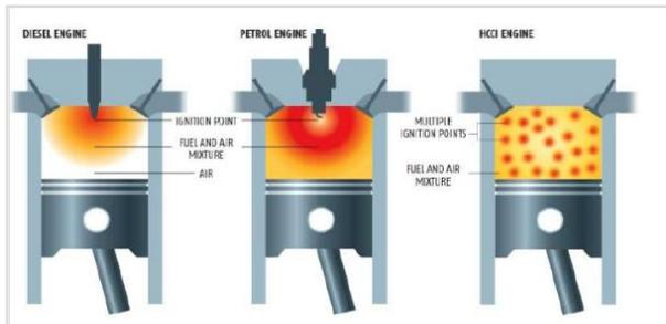
Figure 1.1 Three modes of Combustion
