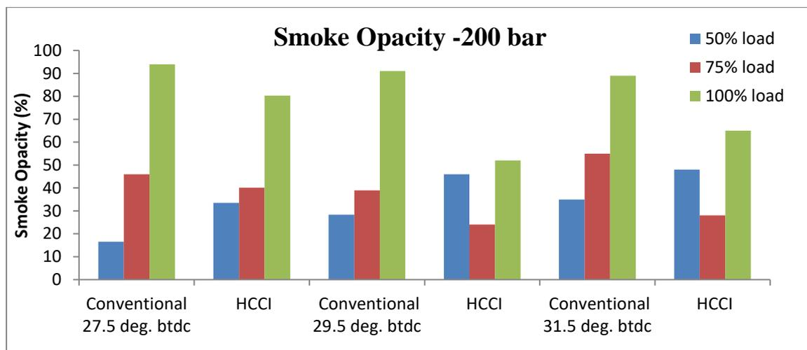
Figure 4.4.2 Smoke Opacity for conventional and vapour induction mode at different injection timings at 200 baR.
