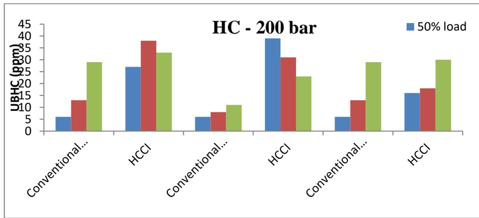
Figure 4.1.2 UBHC emissions for conventional and vapour induction mode at different injection timings at 200 bar
