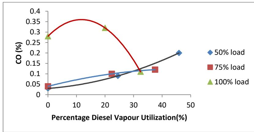
Figure 4.3.3. Effect of vapour induction on CO Emissions at 31.5 deg. btcd and 200 bar injection pressure
