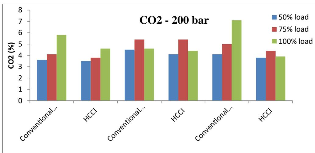
Figure 4.2.2 CO<sub>2</sub> emissions for conventional and vapour induction mode at different injection timings at 200 bar
