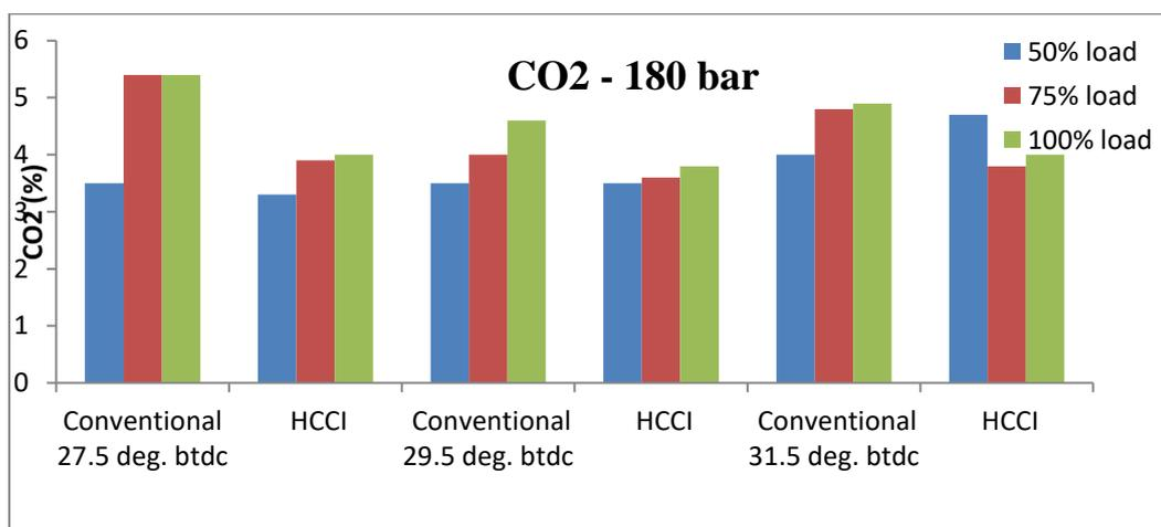
Figure 4.2.1 CO<sub>2</sub> emissions for conventional and vapour induction mode at different injection timings at 180 bar
