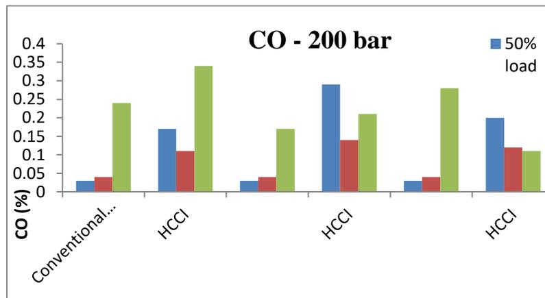
Figure 4.3.5. CO emissions for conventional and vapour induction mode at different injection timings at 200 bar.
