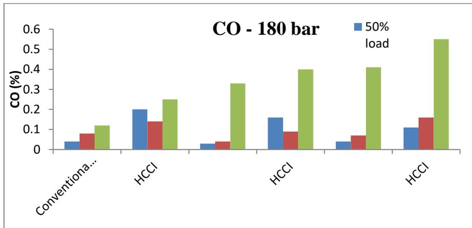
Figure 4.3.4. CO emissions for conventional and vapour induction mode at different injection timings at 180 bar.
