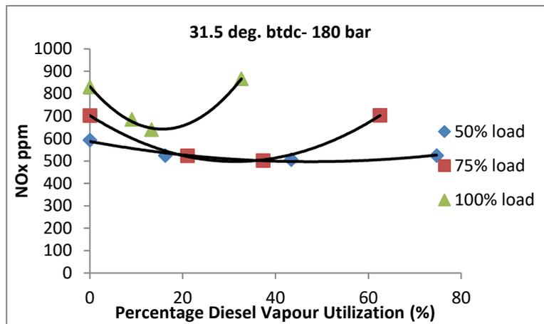
Figure 4.3.3. NOx variation with vapour induction at 31.5 deg. bt dc and 180 bar injection pressure.
