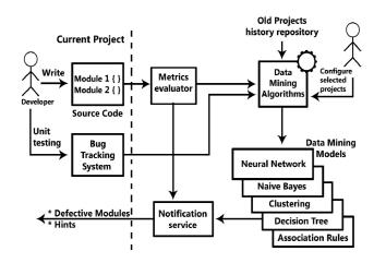
Figure 1. Architecture for defective module identification using data mining and Software metrics<sup>[2]</sup>
